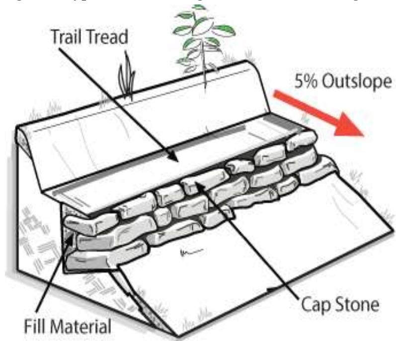
Figure 6: Typical MPOS Design for Natural Retaining Walls
