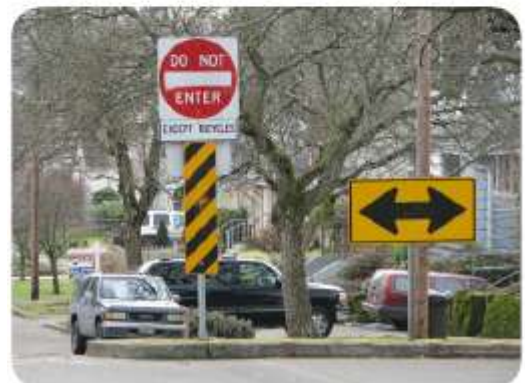
Traffic diverters prevent access to both directions of motor vehicle traffic.
